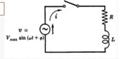
1. Complementary (Transient) Solution is the solution of the homogeneous 1st order DE
